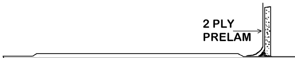
While the spar glass resin is still wet put the ribs into place on the top skin with 5-minute epoxy. Use some small weights to temporarily hold the ribs to the skin until the 5-minute epoxy cures. Run a 1/4 inch micro fillet in each corner of the outboard ribs only.
